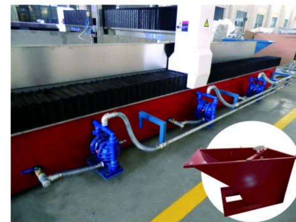
自动清淤系统 Auto Sullage Removal System
