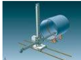
Inner peripheral welding (with the rotator)
