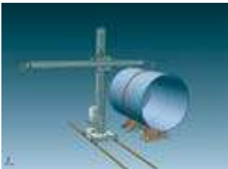
Outer peripheral welding (with the rotator)
