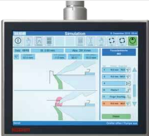
FOLDING SEQUENCE SIMULATION Folding sequence simulation with collision monitoring system for checking programmed profiles.
