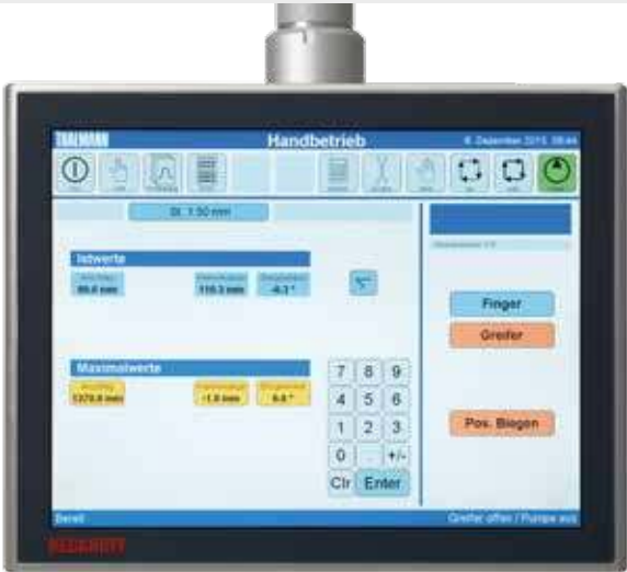
MANUAL MODE The manual mode allows individual folds to be created quickly and without major programming work.
