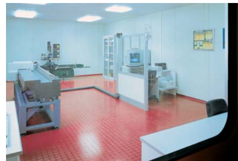
Sala metrologica: le righe ottiche e magnetiche GIVI MISURE vengono testate in condizioni ambientali e climatiche rigorose: T = 20^{\circ}\text{C} \pm 0,1^{\circ}\text{C} U.R. = 45 ÷ 55 % Metrological room: GIVI MISURE optical and magnetic scales are tested in rigorous environmental and climatic conditions: T = 20^{\circ}\text{C} \pm 0,1^{\circ}\text{C} R.H. = 45 ÷ 55 %
