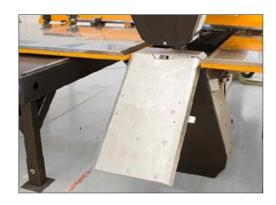
Frontal reclining table for unloading the workpieces
