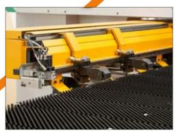
Automatic and programmable sheet metal locking clamps
