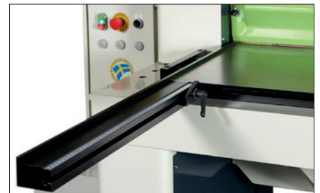
Equip your sheet metal shear with a long squaring arm (up to three meters), and add a T-groove and tilting stop.
