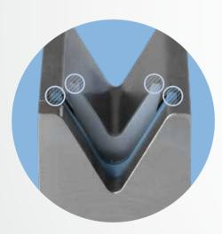
The heart of the system is the **double-fork-sensor** establishing **4 contact points** on the material: this detects the bending angle on two points on both sides of the bend. It then sends the data to the control system, thus enabling a perfect bend angle from the first piece to the last.
