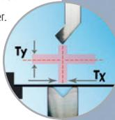
**F** Tool Holders suitable for 'Shoulder' load New Standard and American Style bottom tools with NS V and VI adaption.
