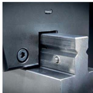
E2M® top tools are provided with bearing safety pins in the adaption of the tool. Applicable for: head and shoulder load top tools with a minimum tool length of 100mm/3.397". Tool weight should be between 12.5kg/28lbs and 100kg/220lbs.
