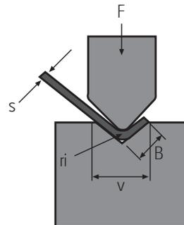
F = Tons per meter of workpiece
