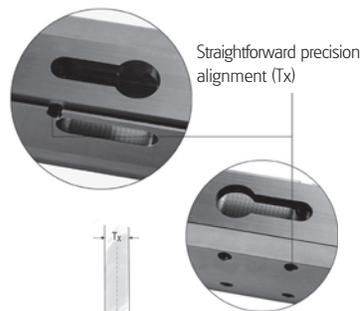
Tx-adjustment is needed to configure the position of the bending line (centerline of tools) in relation to the back gauge of the press brake, to an extremely high level of precision. Ideally, all Tool Holders should feature this capability.
