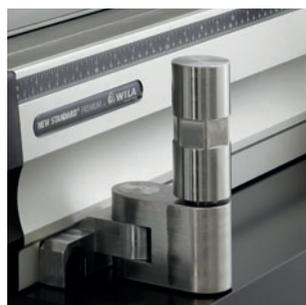
When using "HD" Tool Holders, it is possible to install 'pillars' to further support very wide and heavy bottom tools. These pillars offer additional stability to tools during the bending process. Available every 255 mm/10.039" on front and backside.
