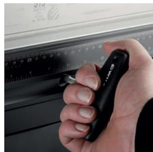
Ty-adjustment is crucial in determining the parallelism between top and bottom tools. Adjustment in Y direction makes it possible to fully compensate for unavoidable - cumulative - processing tolerances in the press brake. Either the top or bottom Tool Holder must be able to do this if one wants to achieve accurate and consistent bending results.
