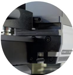
*Each upper Tool Holder, used in combination with a Press Brake Productivity ToolStation, requires a dedicated guard with a safety mechanism for safe loading and unloading of the top tools (with E2M<sup>®</sup>). The movable load/unload arm will lock and unlock the guard.*
