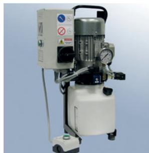
For use in combination with Tool Holders with Hydraulic Clamping. Operation via push button on the power pack, via remote control, or fully integrated in the press brake. See also page 131.
