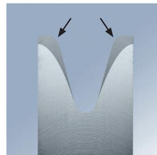
New Standard Bottom Tools in the OZU-3\*\* and OZU-4\*\* series feature extra large shoulder radii (R = approx 20% of V-opening) which greatly reduce part marking during the bending process.
